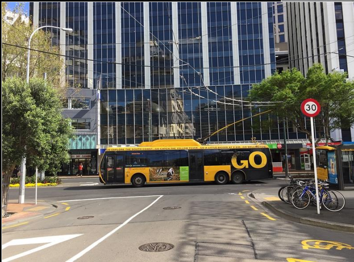
Right: 357 was photographed at the north end of Lambton Quay on 10 October on a Route 2 working to the Railway Station. The bus is about to travel through the cross over special work at this location with the driver getting a prompt on the roadway ahead of him.
