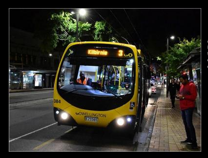
*Right:* With its last journey almost over and 384 now in Onepu Road by the Pak 'n Save supermarket, a request was made to the driver to drop the poles and have the bus travel on battery power for the last 100m or so to the depot. Under the circumstances the driver was happy to oblige. Photo: Ben Foden.
