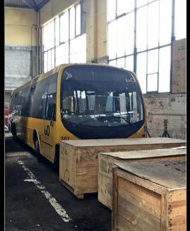
Above: 376 (and all its colleagues) have been earth tested for the very last time. From now on they will either have to be moved using their onboard battery power (for how long that lasts) or be towed by the depot tractor. The electricity to the overhead has been switched off.
